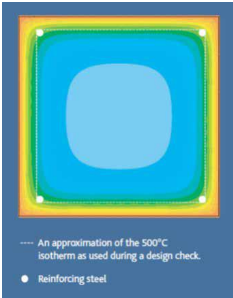
Design of RCC in fire
