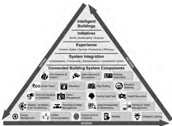
Figure 2: This diagram illustrates the process of defining and designing the building systems and components that deliver on the stakeholders' vision of a truly intelligent building. It is a visual representation of the process to define the client's goals and initiatives for an intelligent building.
