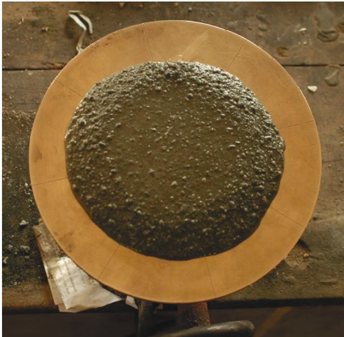
Fig. 3 – M-sand mortar at 85% flow (no segregation)
