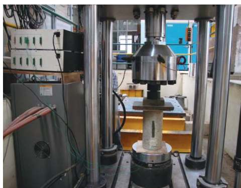
Fig. 9 – Test set-up for stress-strain measurements and the failure pattern of concrete cylinder
