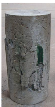
Fig. 9 – Test set-up for stress-strain measurements and the failure pattern of concrete cylinder
