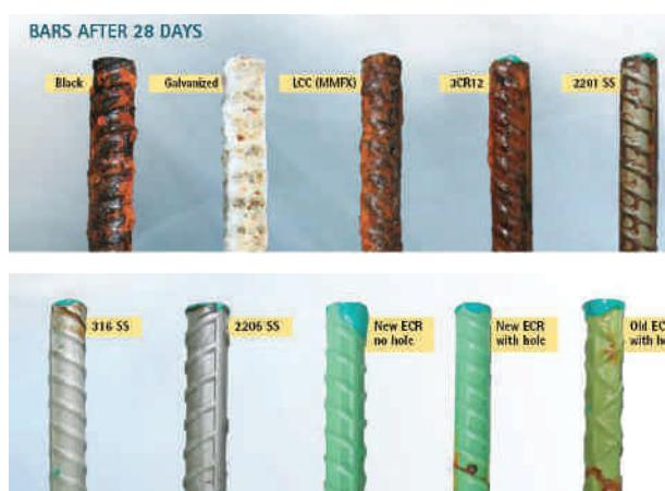
per year is the lowest for fusion bonded epoxy coated steel without holidays.
