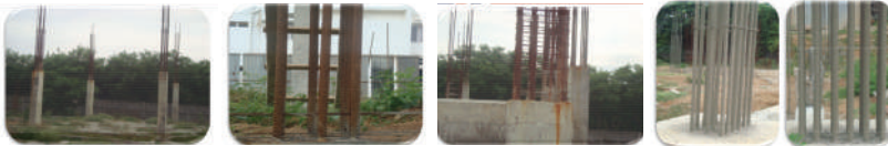
CPA coated bars after 8 months marine exposure at Muttukadu, Chennai
