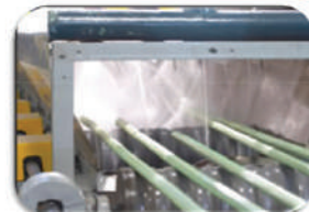
Epoxy Coating – Electrostatic Spray Technique
