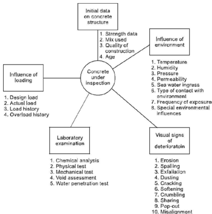
Fig. 12 Concrete investigation method
