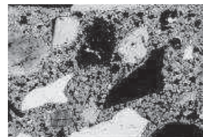
"Pop-corn" like calcite crystals present in carbonated paste. The concrete is suffering from bi-carbonation.
