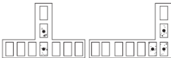
Fig. 26.15 Vertical reinforcement in cavities for hollow block masonry
